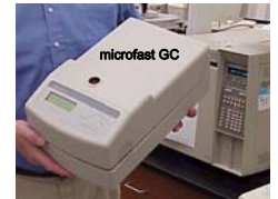
microFast GC: portable, extremely fast, runs on a 12V/24V battery
