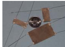
Metal tubing attached to the nickel columns using a silver paste which can withstand 300 C
