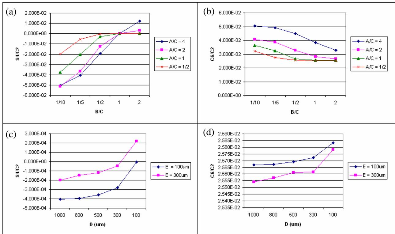
Figure 2 – Simulation results with electrodes only (a) First odd higher-order component  $S_4/C_2$  (b) First even higher-order component  $C_6/C_2$ ; Simulation results of optimized electrode geometry ( $A = B = C$ ) with housing (c) First odd higher-order component  $S_4/C_2$  (d) First even higher-order component  $C_6/C_2$
