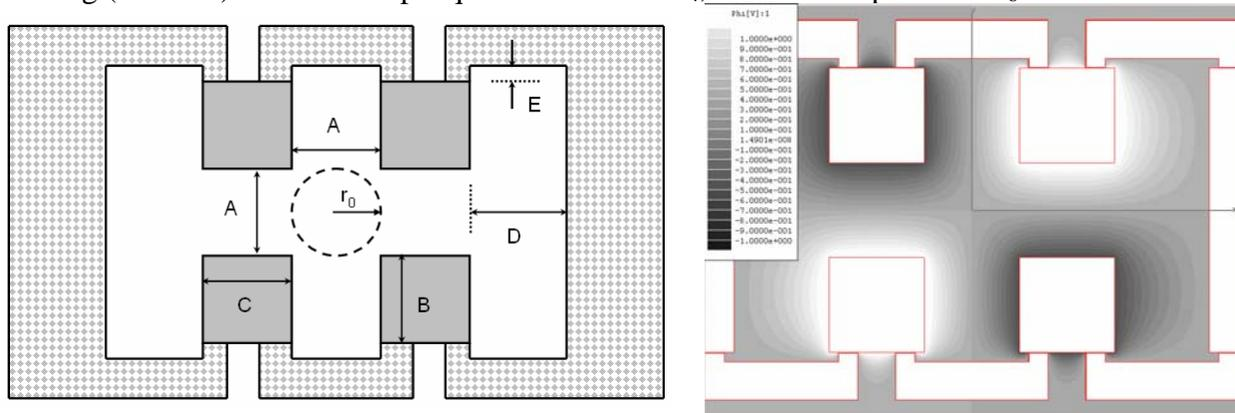
Figure 1 – (left) Cross-sectional view of device geometry used in simulations (solid: electrodes, textured: housing). Dimensions A-E are parameterized and  $r_0$  is the effective device aperture radius; (right) Maxwell-3D potential field solution for a specified geometry
