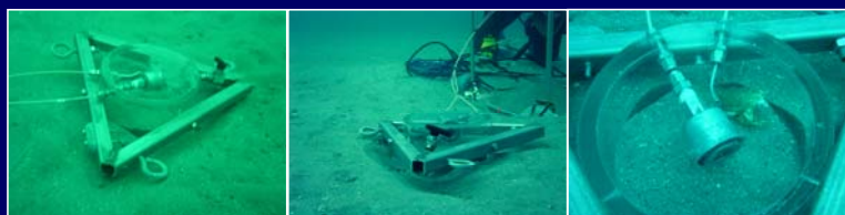
Mass Spectrometry Deployment - The mass spectrometer was lowered overboard to the seafloor by the ship's winch. The benthic chamber was deployed into the sediment by divers. Divers also connected the power, communication tether to the mass spectrometer.
