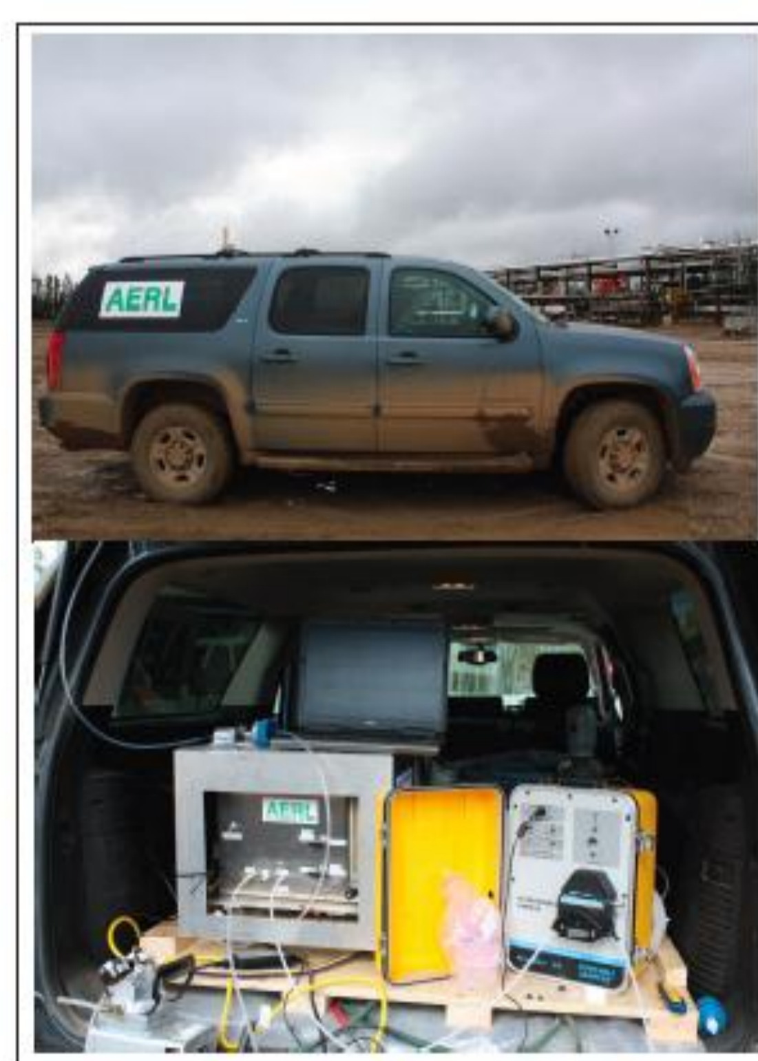
Figure 2. The MIMS system continuously analyzing aqueous sample from an on-site creek.
