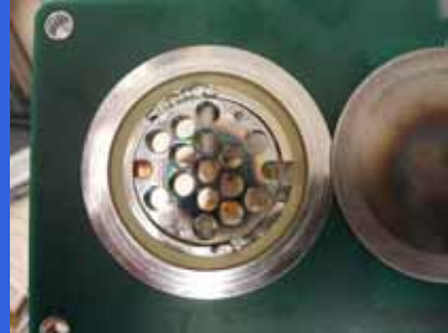
PCB artwork for ion sputtering pump showing multi-cell anode plate and one of two cathode disks (2013)
