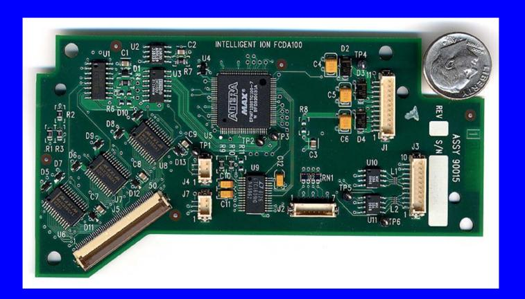
The multiplexing and integration board sits in the vacuum housing
