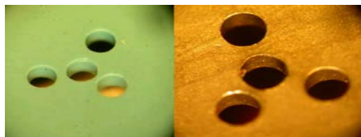
Figure 3. On the left, holes are drilled in the laminated green tape before firing at 850°C. Lamination of green tape sheets allows for various thicknesses. On the right, electro-less nickel is applied to the laminated and fired green tape structures.
