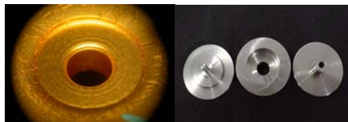
Figure 4. On the left, a CIT is fabricated by compressing green tapes in a die. After firing at 850°C, the CIT is first plated with electro-less nickel and after that with electro-less gold. Shown on the right is the stainless steel die.
